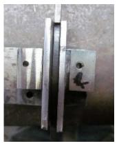
Go to the anvil and set the rivet. If all is well, the bolsters are now level with the shoulders of the tang, are parallel to one another and are locked down to the blade. Remove excess JB Weld with acetone, paper towels and the edge of a tongue depressor (or Popsicle stick). Don't forget to clean the alignment plates.
