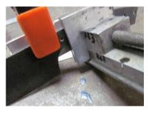
Position the correct block (here the right side one) with the polished face forward and the milled angle face to the blade and use a transfer punch to mark the location for the rivet hole.
