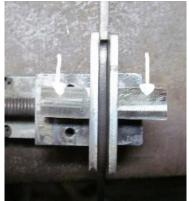
It is a good idea to chamfer the outer end of the hole to allow the rivet to spread and lock the blocks down when the rivet is hammered.
