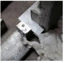
If needed, grind off any rivet that protrudes and clamp the blade in a decent vise as shown. Depending on air temperature, expect to wait until the next morning before moving onto the pommel & handle tasks.
