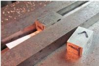
To check, assemble the blocks in position and measure the total thickness top & bottom. Here, it is off by 5 thousands.
